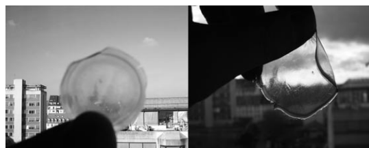
Figure 3. Thin films based on Diels–Alder chemistry, obtained by blending a) 2 (1 equiv), 8 (0.6 equiv) and 10 (0.2 equiv) and b) 2 (1 equiv), 8 (0.8 equiv) and 10 (0.1 equiv).
